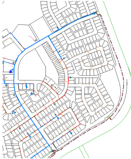
Figure 4: Old 35 kV Looped Configuration
