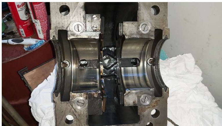
Figure 6: Turbine Journal Bearing Minor Wear
