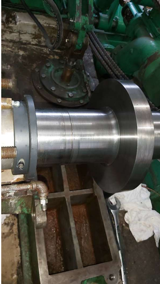
Figure 5: Turbine Journal Bearing Shaft Scoring
