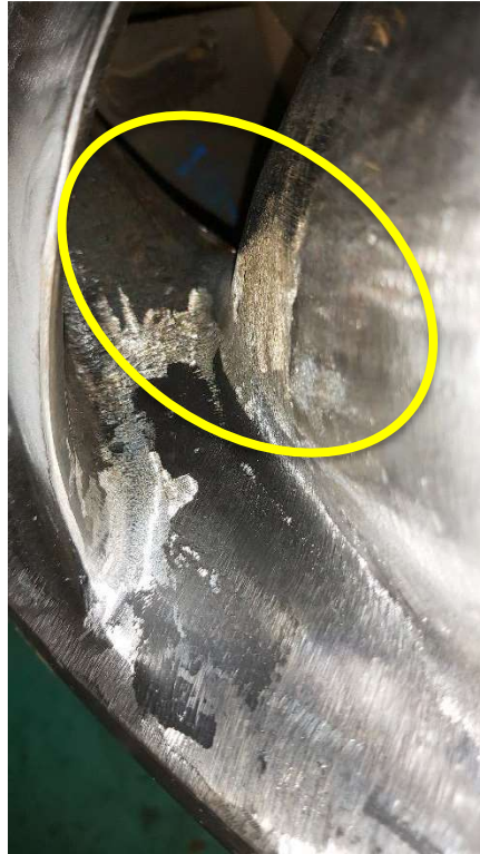
Figure 2: Runner Suction Side Cavitation (expansion too severe)
