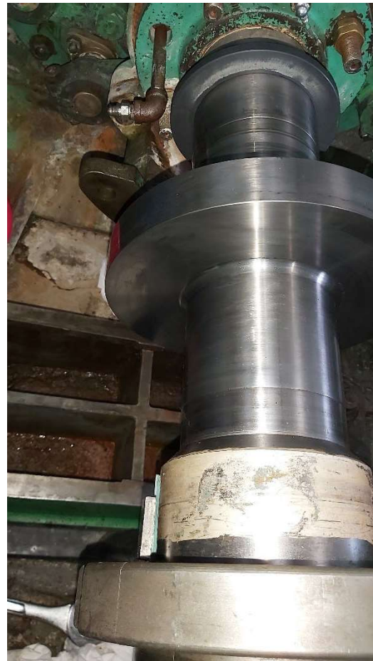
Figure 5: Turbine Journal Bearing Shaft Scoring
