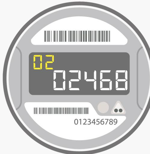
**02** indicates the amount of **kWh** that is being redirected back to the grid.
